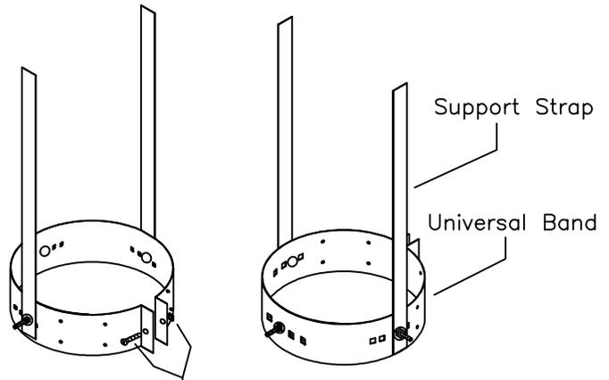
Fig 2 1/4" x 2" ss screw and nut through tabs
