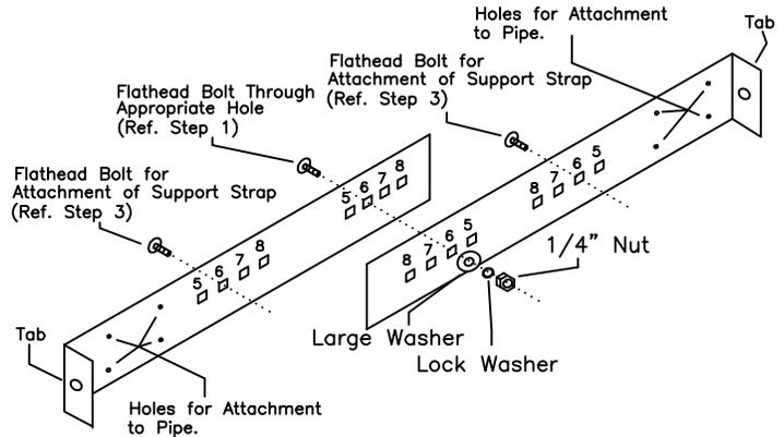
Universal Wall Band (Fasteners oriented for 6" system)
