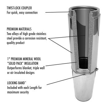
\*NOTE: 4" diameter slightly different - no locking band required. See installation instructions for more details.
