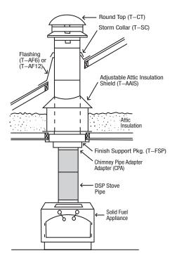
3. Wood Heater with its chimney through an upstairs enclosure
