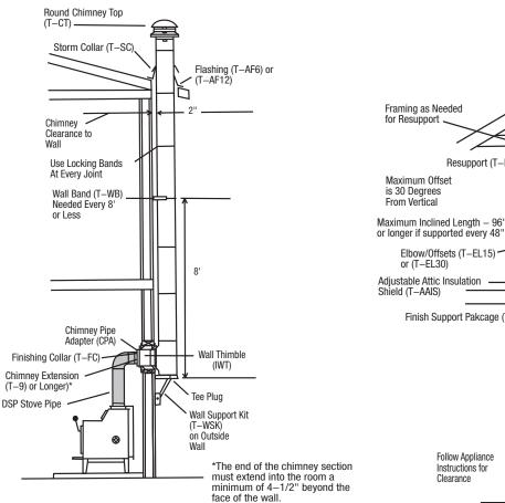
5. A-Frame with chimney on a steep pitch roof
