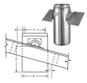
Note: \* An 18" Chimney length included with RSP Roof Support Package. \* Framing dimension for the installation of the RSK is identical to the RSP dimension. "t" varies with slope.
