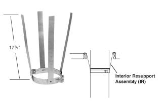
• Incorporates the flexibility to work on 5", 6", 7" and 8" diameters and is an excellent method for resupporting chimney systems that have offsets or vertical runs that require additional support (up to 18 feet).
