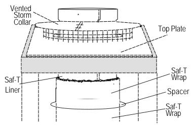
The following instructions are additions or alterations of the Saf-T Liner Installations & Maintenance Instructions and are not intended to be exclusive. To insure a safe and proper installation, follow the procedures in the enclosed Saf-T Liner Installation & Maintenance Instruction manual. Note: This system may be used to vent the flue gases of UL or other Listed appliances, with maximum continuous flue-gas outlet temperatures not to exceed 1000°F.
