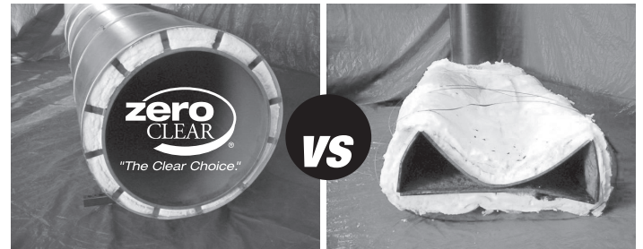
ZeroClear® after 2000°F (simulated grease fire) for 30 minutes.
