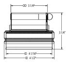
• Used on appliances with a thicker flue outlet collar.
