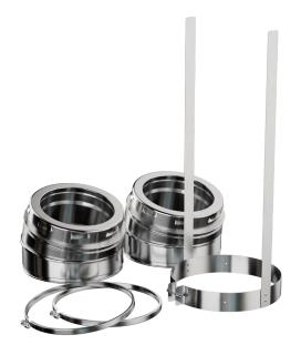
15° Insulated Elbows can be used for fixed offsets of 15° slope or in pairs for offsets adjustable from 0° to 30° slope. The 30° Insulated Elbow in 5", 6", 7" and 8" sizes can be used for fixed offsets of 30° slope. Greater angles are prohibited by UL® Standard 103 and by the terms of the product listing.
