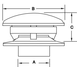
**Note:** The 10" diameter Round Top is designed with a squeeze collar that fits inside the chimney pipe and a set screw which is tightened to hold the top firmly in place.
