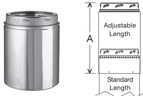
**NOTE:** Adjustable Lengths must be installed above a fixed length - they cannot be installed immediately above a support, tee or elbow.
