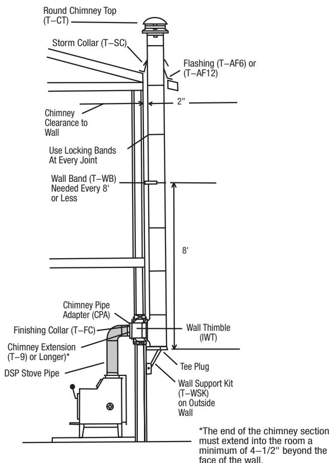
**5. A-Frame with chimney on a steep pitch roof**
