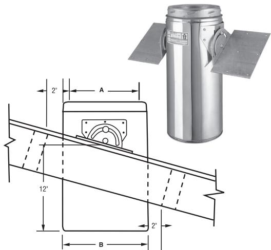
**Note:** \*An 18" Chimney length included with RSP Roof Support Package.
