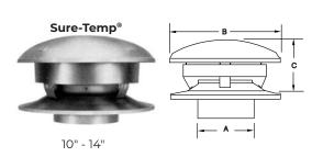
Note: The Round Top for 10" to 14" diameters is designed with a squeeze collar that fits inside the chimney pipe and a set screw which is tightened to hold the top firmly in place.
