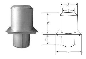
The Attic Insulation Shield is used wherever the chimney enters an open attic. A drop-down Joist Shield is included for use when the chimney is enclosed below the ceiling. Refer to instructions for full details. The Attic Insulation Shield acts as an insulation shield to keep blown in or blanket insulation from filling in any framed opening or contacting the chimney.
