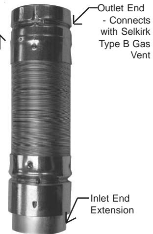
To install: Extend inlet end down over collar of appliance draft hood and secure in place with minimum 3 screws (not supplied) through the inlet end extension of the EFC and the collar of draft hood (see Figure 3). With the EFC Inlet End secured to the draft hood, extend the EFC to the required length and secure the Outlet End of the EFC to the inlet end of the Type B Gas Vent.
