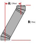
A maximum of two offsets (4 elbows in all) is allowed per chimney system. The chimney must not be inclined more than 30° from vertical in the USA and 45° in Canada. Offset charts are available to assist in determining your offset and rise.
