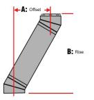
A maximum of two offsets (4 elbows in all) is allowed per chimney system. The chimney must not be inclined more than 30° from vertical in the USA and 45° in Canada. Offset charts are available to assist in determining your offset and rise.
