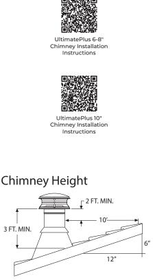
Note: The chimney must extend at least three feet above the highest point where it passes through the roof surface and at least two feet higher than any part of the building within a horizontal distance of ten feet.
