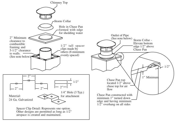
NOTE: Chimney outlet to extend a MINIMUM 6" above Chase Pan. 2" MINIMUM clearance is to framing only.
