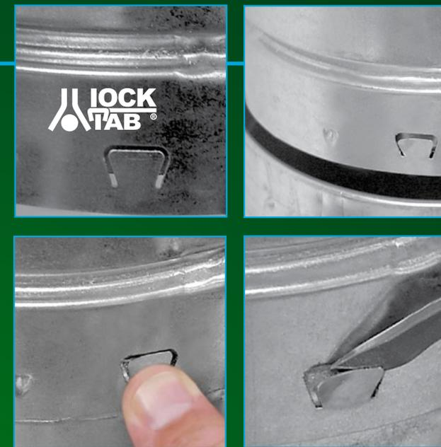
*Locks together with a snap, allowing you to engineer the perfect application. To disassemble - simply rotate the pipe, align the dimples, and pull apart.*
