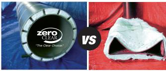
**ZeroClear**<sup>™</sup> after 2000°F (simulated grease fire) for 30 minutes.
